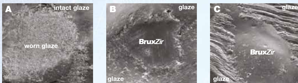
It is apparent that glazes used on all the crowns in this study will not be long lasting. Image A shows glaze disruption to e.maxCAD by a ceramic onlay; Image B shows glaze worn off a BruxZir cusp tip by opposing cast gold; Image C shows where occlusal adjustment stripped away the glaze and left the zirconia underneath untouched.
